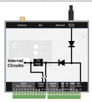
All the terminals marked with a ground symbol are electrically connected together internally. This is also the same ground as the sleeve of the barrel jack, and the antenna connector.
