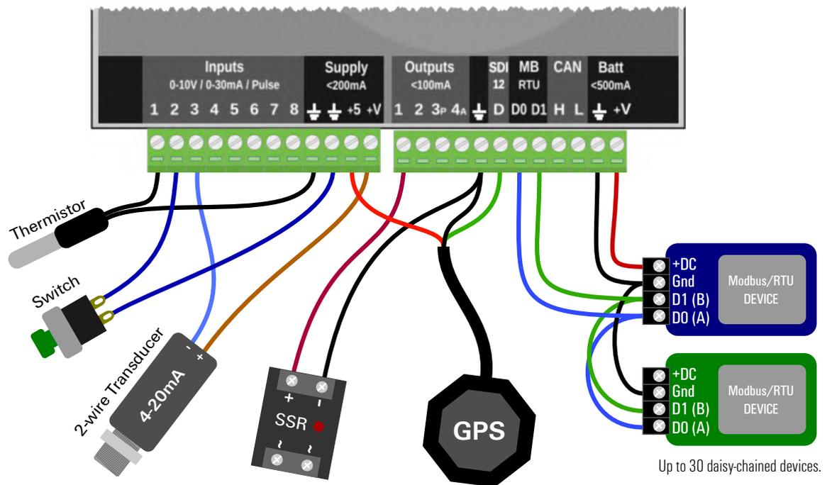
This shows a small selection of common devices and how they can be connected. Please refer to [doc.eze.io](http://doc.eze.io) for more details on these and other types of connections.
